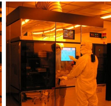
Ultratech XLS 200 4X reduction stepper 0.5 \mu m resolution
